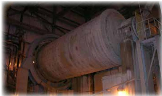
herringbone gears. The size of the bull gear will usually range from 1.8 to 12.2 meters (6 to 40 feet) in diameter. The pinion gear normally varies from 1/2 to 3/4 meter (1-1/2 to 2-1/2 feet) in diameter. Although various drive configurations exist, the pinion is usually driven by an electric motor through a gear reducer. Pinion speeds range from 15 to 250 rpm, and bull gear speeds are approximately 20 rpm, depending upon the inside radius of the rotating drum.
