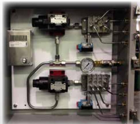
Farval reports that asphaltic products can harden in the lube lines and valves, which can cause lubricant starvation. If this situation is not detected before damage occurs, catastrophic failure can result. The close tolerance
