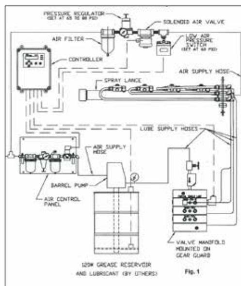
**Above:** This Bijur Delimon Singline model is a typical automatic spray lubricating system, with pump close to valve panel. **Below:** A Bijur Delimon system "in a box" for customer demonstrations.
