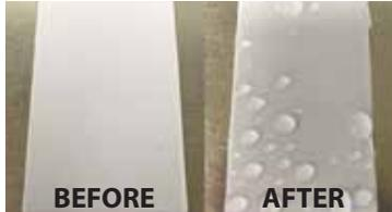
**Water Resistance** – Incorporated into LE lubricants, Quinplex helps form a water-resistant barrier and prevent water spray-off loss, which means fewer equipment failures caused by a lack of lubricant. It also means longer regreasing intervals and less lubricant usage.
